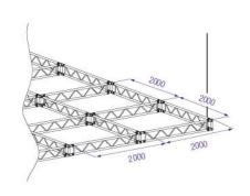
Spans must be supported at each end.
