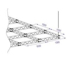
Spans must be supported at each end.
