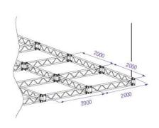
Spans must be supported at each end.
