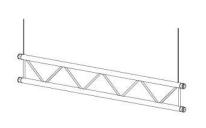
Spans must be supported at each end.
