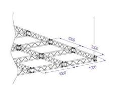
Spans must be supported at each end.
