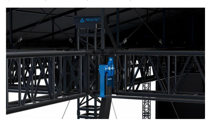
Increased cantilever design provides extra depth to your performance stage area. The impressive front extension has the full loading capacity of normal spans. This offers your audience a clear and wider unobstructed views.
